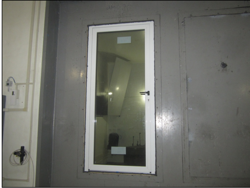
Receive Room View of Installed Test Specimen
